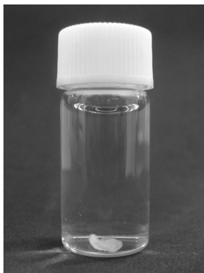
Fig. 1. Photograph of PWA-conjugated chitosan matrix (chitosan:PWA = 10:100) in aqueous solution.
